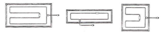
7. Note that more cable is used around the perimeter and less in the center of any pattern. This will create a more uniform temperature throughout the planting area. An exactly uniform cable pattern will produce a warmer center and cooler perimeter all around. The depth of burial and moisture content of soil will also affect temperature uniformly.
