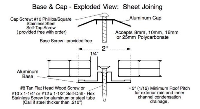
Base & Cap System<sup>™</sup> placed on placed on vertically running rafters and studs (below). Dimension from outside of structure to center of first or last framing member and Base is 48-1/2", less if using Roof Corner Overhang Detail. On-Center dimension between Intermediate framing members and Base is 49". Use spacer if high humidity.
