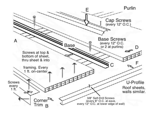
Structural Loads & Special Screw Postioning for High Wind Areas.
